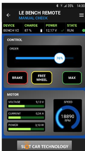
In the **CONTROL** section, the slider allows you to adjust the engine setpoint manually. The **BRAKE** button stops the engine with maximum braking, the **FREE RUNNING** button stops the engine coasting. The **MAX** button sets the engine setpoint to 100%.
