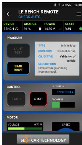
The **SIMU DRIVE** test verifies the vehicle's dynamic behavior by simulating driving on the track and performing a succession of laps.
