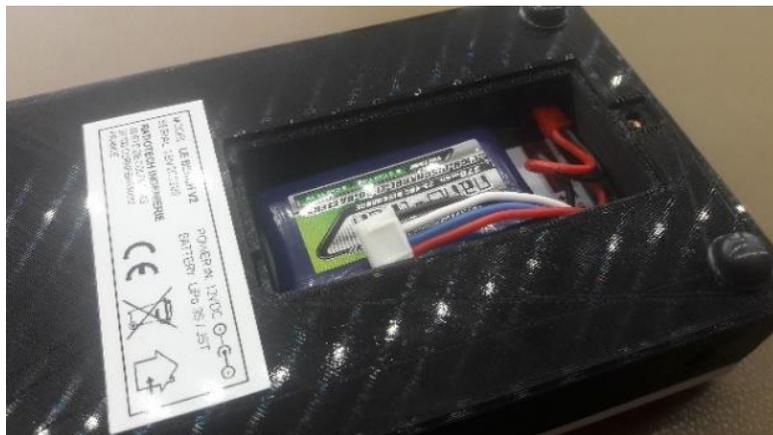
Put the hatch in place on the Bench V2 and then screw in to keep the hatch in position.
