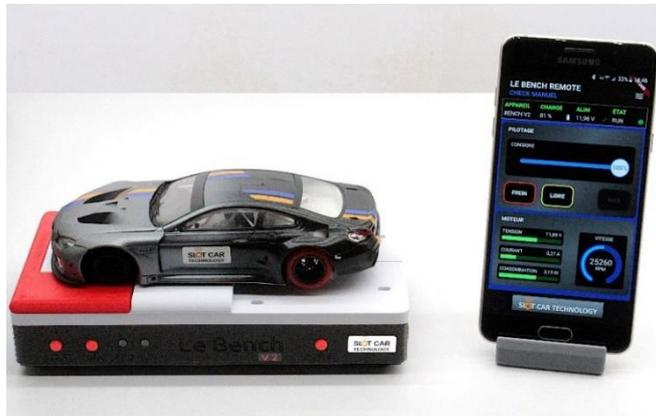
It powers the electric motor of the car being tested and measures the voltage supplied as well as the current and power absorbed. **The Bench V2 also measures the rotational speed of the motor**, without sensor, thanks to a proprietary algorithm offering an accuracy of 0.1% of the measured value over the interval **3,000 to 50,000 RPM (rotations per minute)**.
