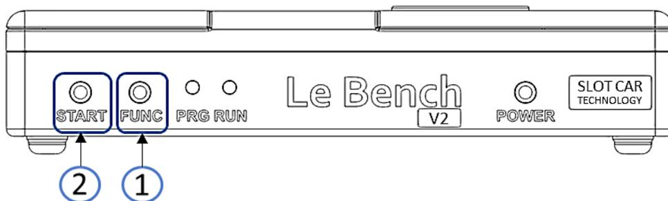
The PRG and RUN LEDs flash 3 times and then turn off, indicating the stop of the Bench V2.
