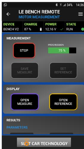
To start measuring a motor, press the **START** button. The measurement stops automatically after exercising the engine in steps of 5% increase in rpm.
