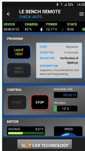
The **LIGHT TEST** is used to check the lighting of the vehicle under test: brightness, holding time, behaviour in the event of a runway departure.
